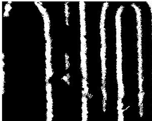
Figure 19. Binary image of detection site; the black indicates the S - shaped channel and reference channel while the white indicates the walls of the microfluidic chip
