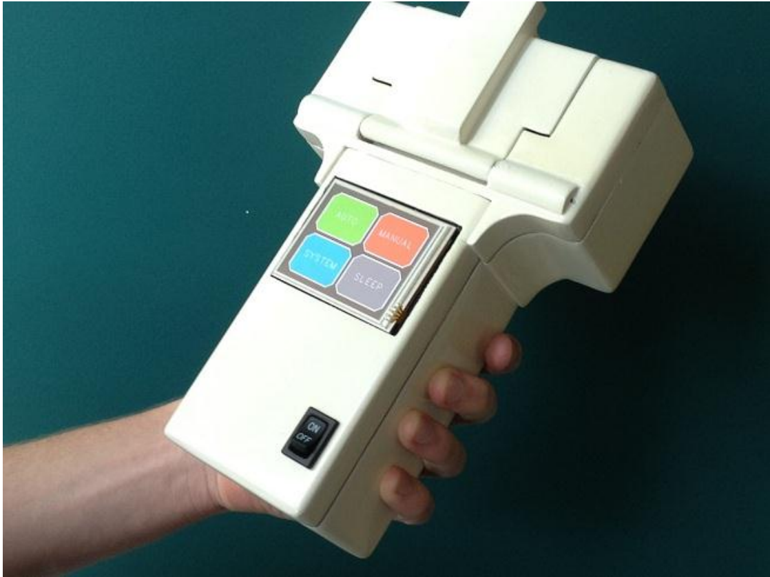
Figure 51. Hand-held lens-less POC LOC device
