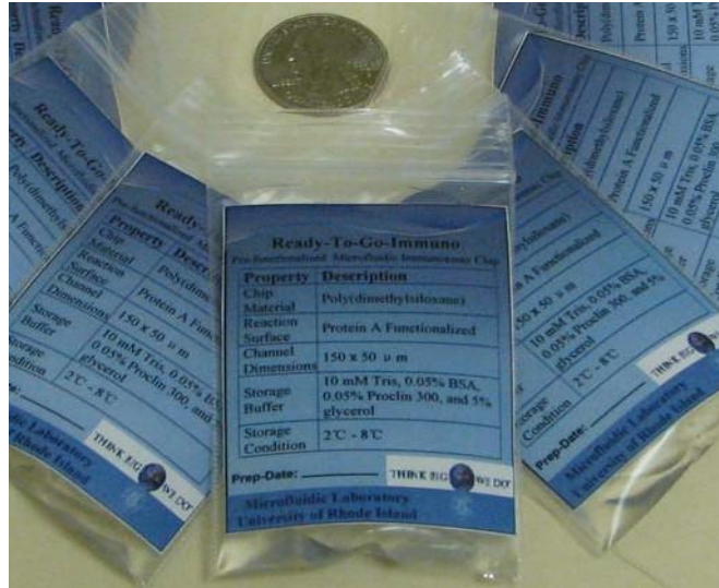
Figure 50. Pre-functionalized ready to run CRP test in vacuum sealed bags
